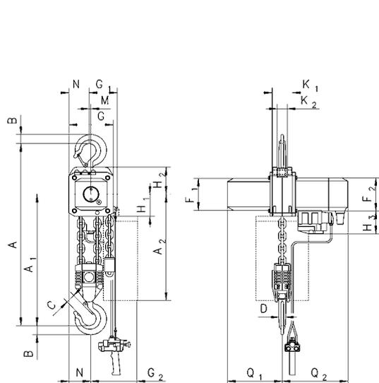
Model CPA ATEX with suspension hook, 4000 - 5000 kg, double fall
